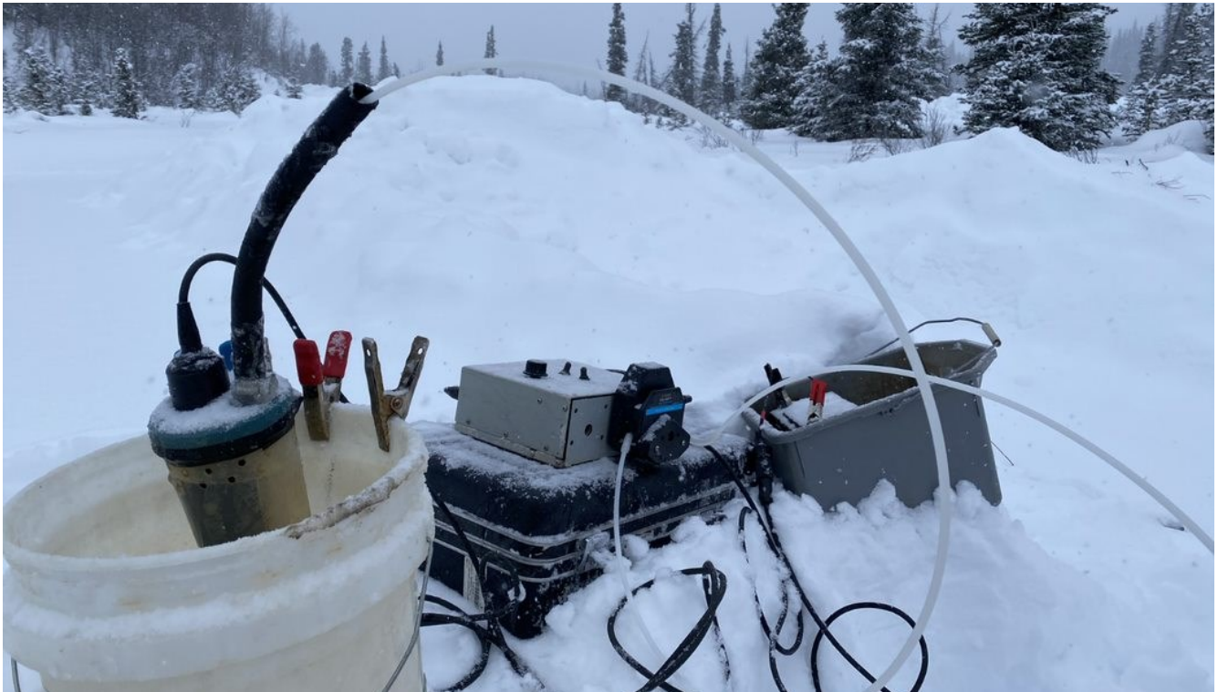
A lowflow peristaltic pump used to collect a groundwater sample at Faro.
